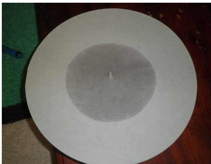
Fig 1. Wicking of filter paper with Silver Nitrate.
