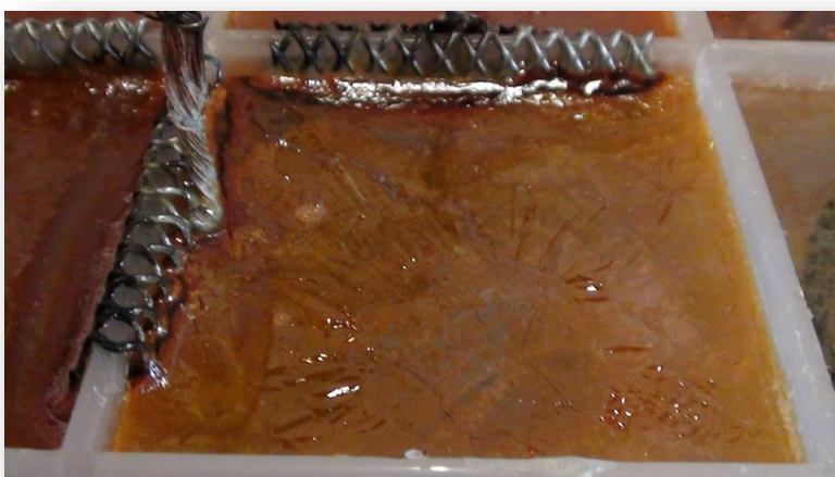
Figure 1: Gans production cell with thick surface layer.
