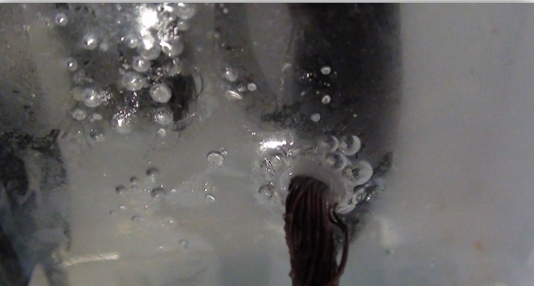
Figure 4: Gans production cell with thick surface layer and gas bubbles
