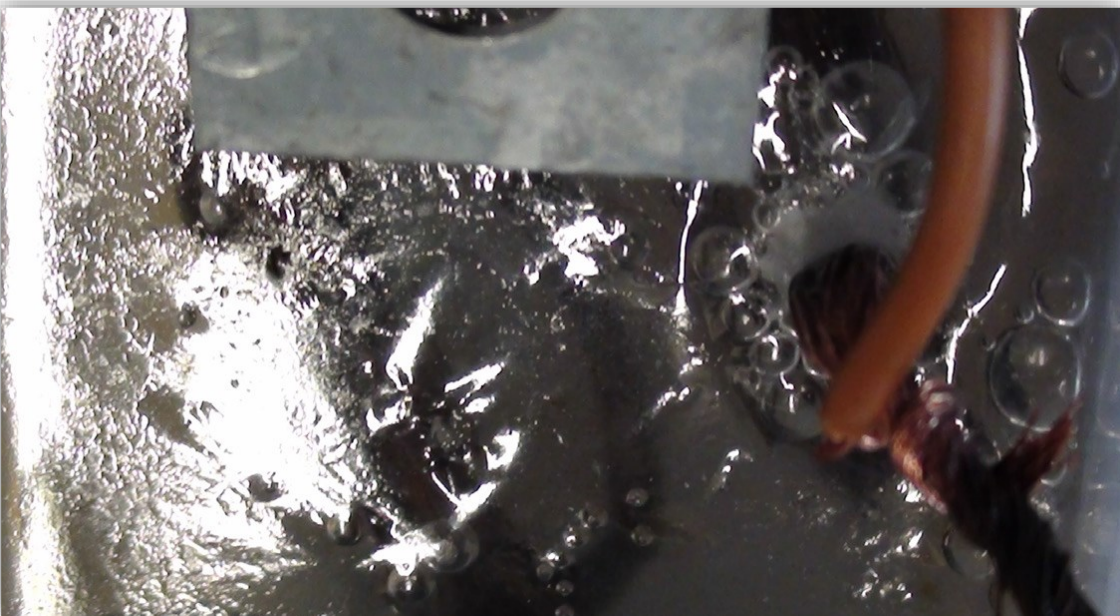
Figure 3: Gans production cell with thinner surface layer and gas bubbles
